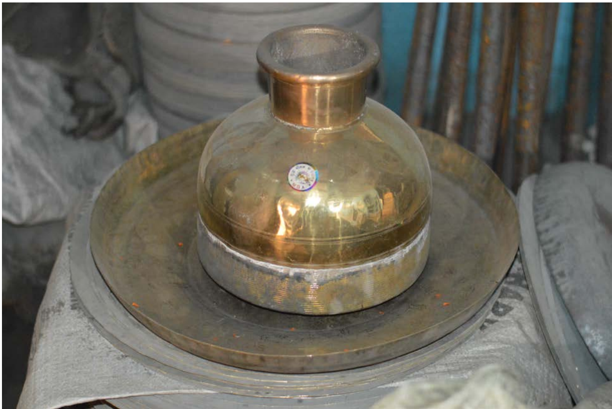
Figure 54 A semi finished brassware utensil
