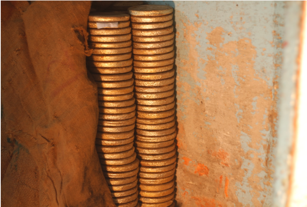
Figure 53 Billets of raw brass. Sheets are prepared from these discs for further shaping
